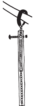
Figure 7. Small-diameter PVC encases a garage door spring to prevent a tiger's claws, lips, etc. from becoming trapped in the spring. The PVC is twice the length of the spring so that even if fully extended, the spring is entirely inside the PVC (Hare and Jarand, 1998).
